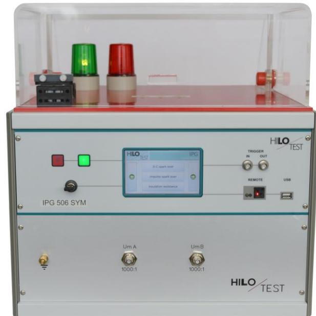
The front-chopped-wave generator IPG 506 is used for measuring dc spark-over voltage and impulse spark-over voltage of over-voltage protectors according to CCITT / ITU-T, K12.
