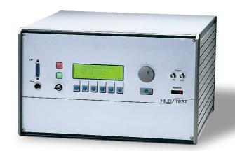
The surge current generator PG 2-750 delivers pulse currents with the waveform  $10/160\mu s$  and  $10/560\mu s$ . Optionally an additional waveform,  $10/1000\mu s$  can be integrated. The generator has four or two surge current outputs.
