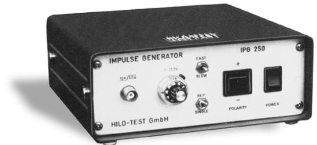
The pulse generator IPG 250 is designed for measuring the step response of high-impedance networks, for instance voltage dividers, oscilloscope probes etc. The generator excels by calibrated adjustment of output amplitude, short rise time and flat pulse top. The output pulse amplitude can be adjusted by use of a 10-turn potentiometer from 0 to 250 V. Positive and negative polarity can be selected.
