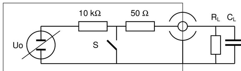
The external load impedance  $R_L$ ,  $C_L$  is connected in series with  $10\text{ k}\Omega$  to a dc-power supply, whose output voltage is adjustable by a precision potentiometer from 0 V to  $\pm 250\text{ V}$ . The make connect switch S short circuits the voltage across the load impedance periodically. During short circuit, the generator's source impedance is  $50\ \Omega$ .
