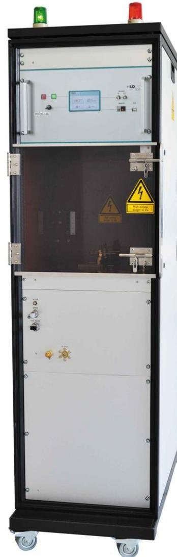
The surge current generators PG20-7000 generates standard impulse currents with waveform 8/20  $\mu$ s according to IEC, EN, VDE. Pulse current output amplitude is controlled by preset charging voltage and can be adjusted up to 50 kA.
