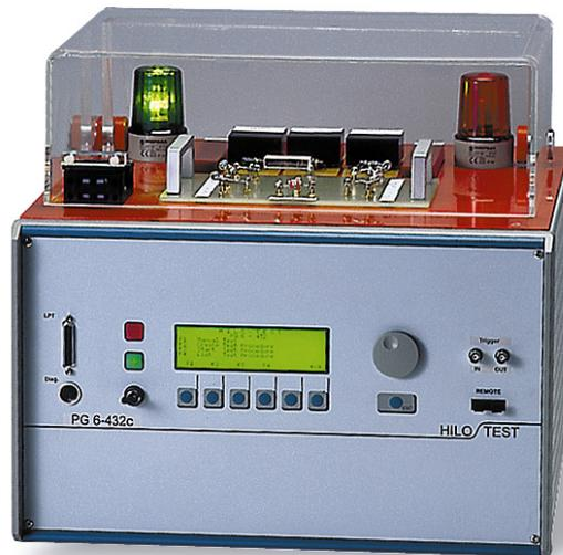
The Surge Test Generator PG 6-432 produces impulse currents with standard waveforms 10/700  $\mu$ s or 10/1000  $\mu$ s. Testing two-gap over-voltage protectors the generator delivers simultaneous at two outputs impulse currents adjustable up to 100 A each. The pulse-forming network contains a high pulse-fidelity current viewing resistor for measurement of the output current amplitude and waveform with a scope.
